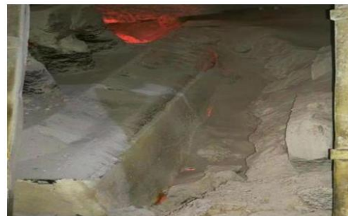
The large face adjacent to the neighboring anode remained unoxidized after 240 hours.
