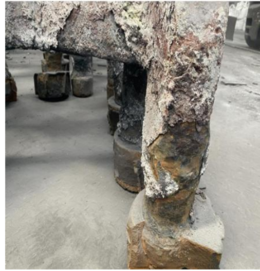
Significant Reduction in Steel Stub Diameter
