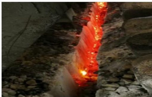
Anti-oxidation protection during preheating of start-up cells
